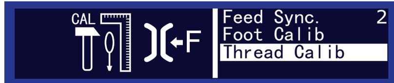
You use this subitem to calibrate the needle thread tension. You will need a thread tension measurement device to perform the calibration (600 g spring balance, part number 0APP 001503).
