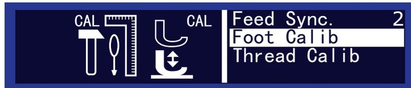
The control must know the upper and lower position of the sewing feet. The upper position is communicated when switching on the machine. The lower position is defined by the calibration performed in this subitem.
