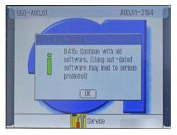
After confirming with **OK**, you can continue working with the old machine software.
