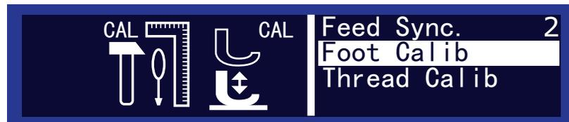
The control must know the upper and lower position of the sewing feet. The upper and the lower position are defined by the calibration performed in this subitem.
