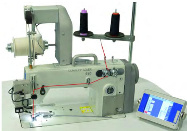
Fig. 7: Threading the needle thread – Part 1
