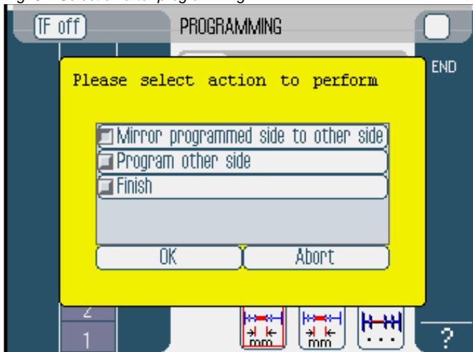
10. Select whether the new seam program is to be mirrored for the other side of the sewing material (Mirror programmed side to other side), programmed for the other side of the sewing material (Program other side) or whether the programming is to be ended (Finish).
