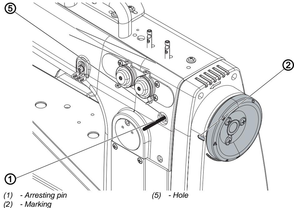
**Locking the machine in place**
