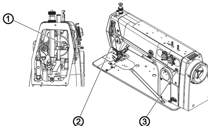
(1) - Slot of arm shaft crank
