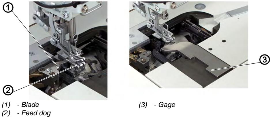
Fig. 38: Setting the looper in the looper mounting (2)
