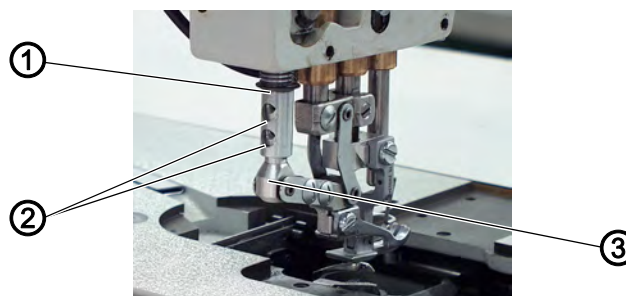
Fig. 59: Setting the position of the top feed foot
