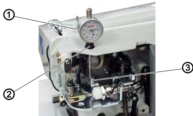
Fig. 33: Setting the needle evasive movement (1)
