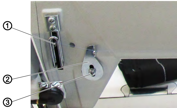
Fig. 71: Setting the thread guide on the machine arm
