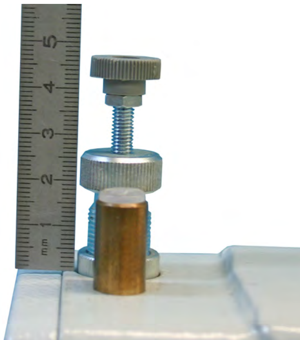
Fig. 76: Calibrating the main feed
