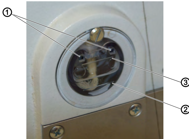
Fig. 77: Lubricating the machine head
