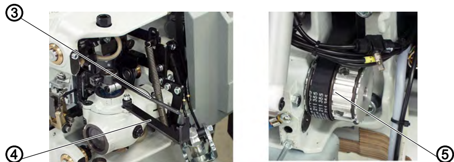
Fig. 37: Setting the symmetry of the looper motion (2)
