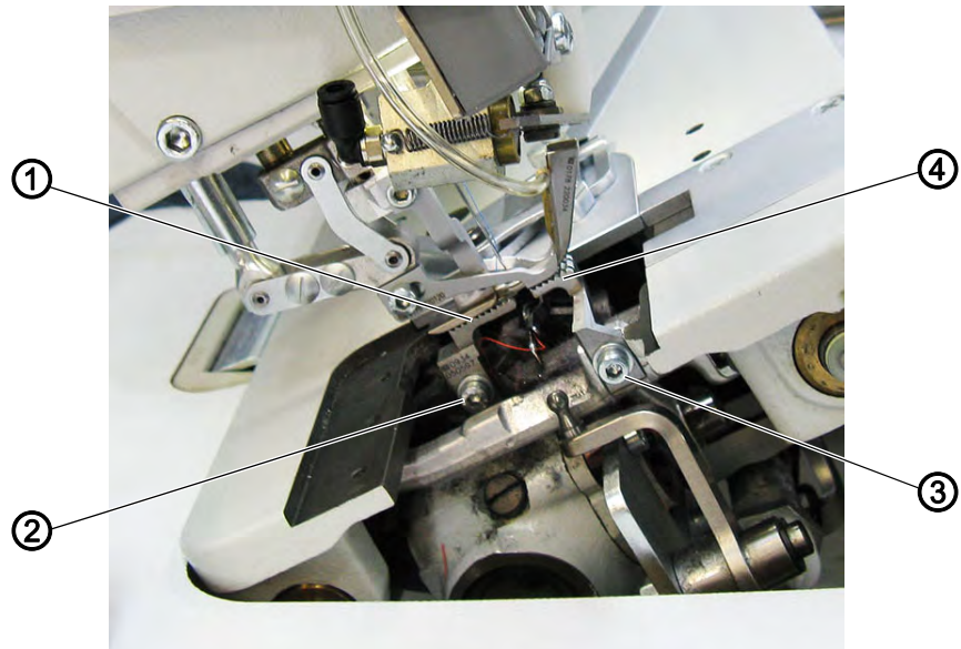
Fig. 7: Removing and installing the feeds
