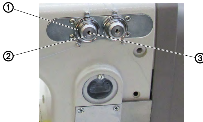
Fig. 75: Calibrating electrical thread tension
