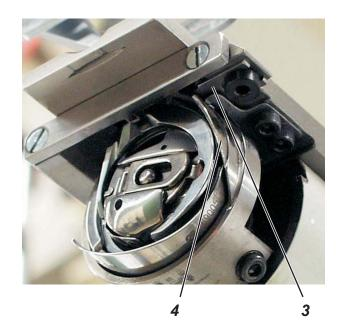
The thread trimmer is switched on electromagnetically.
