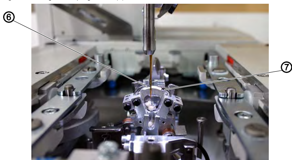
Fig. 67: Setting the looping stroke (4)
