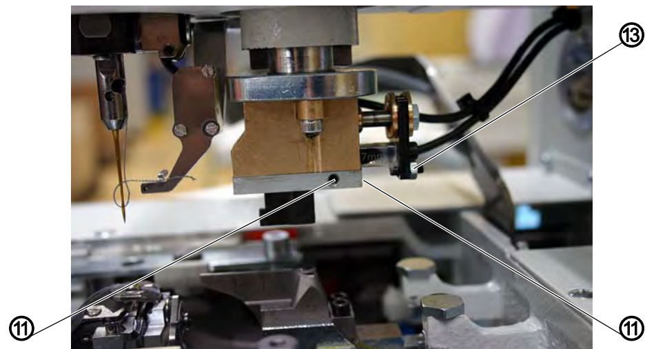
Fig. 56: Setting the cutting block, multiflex (3)
