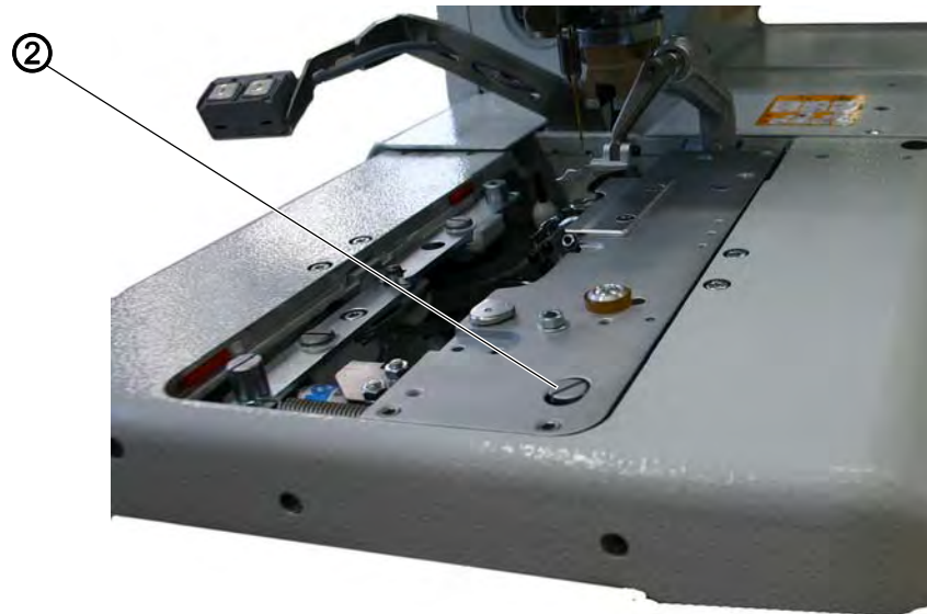
Fig. 29: Aligning the clamping plates (2)
