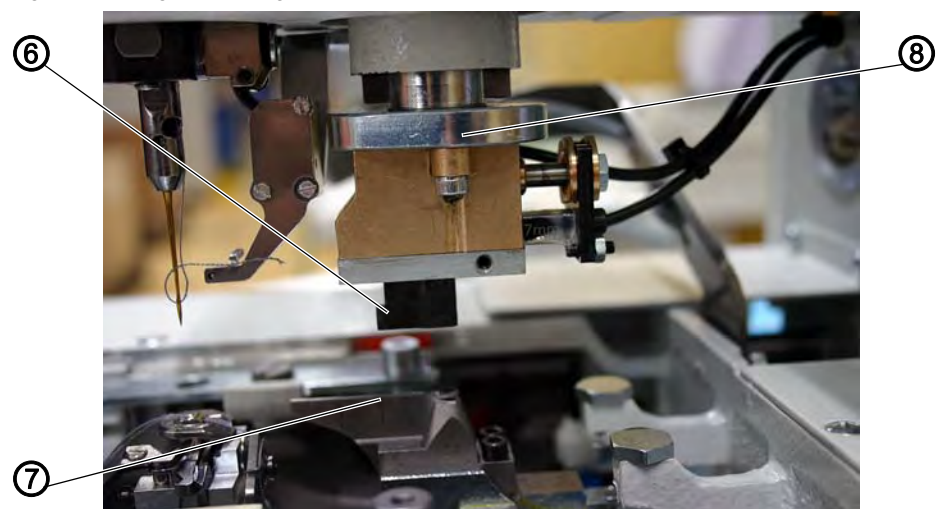
Fig. 54: Setting the cutting block, multiflex (1)
