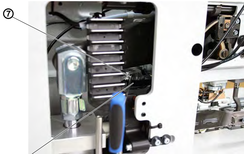
Fig. 19: Aligning the needle bar parallel to the looper turret (4)
