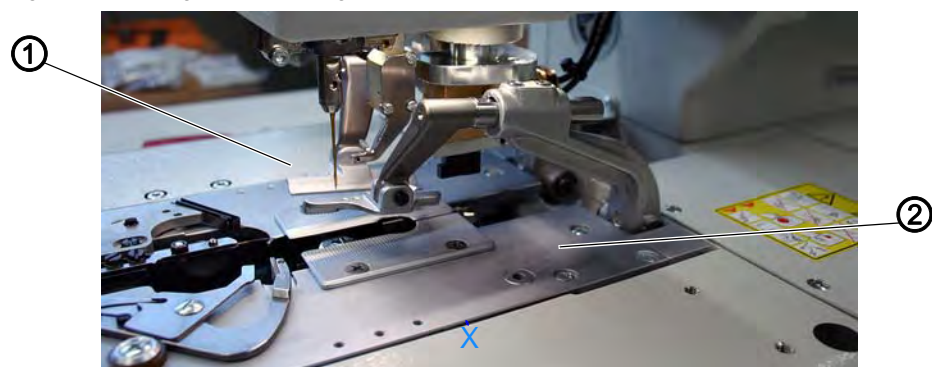
Fig. 30: Clamping plates, setting the spread (1)
