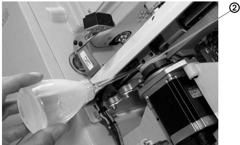
Fig. 170: Lubricating the machine (2)
