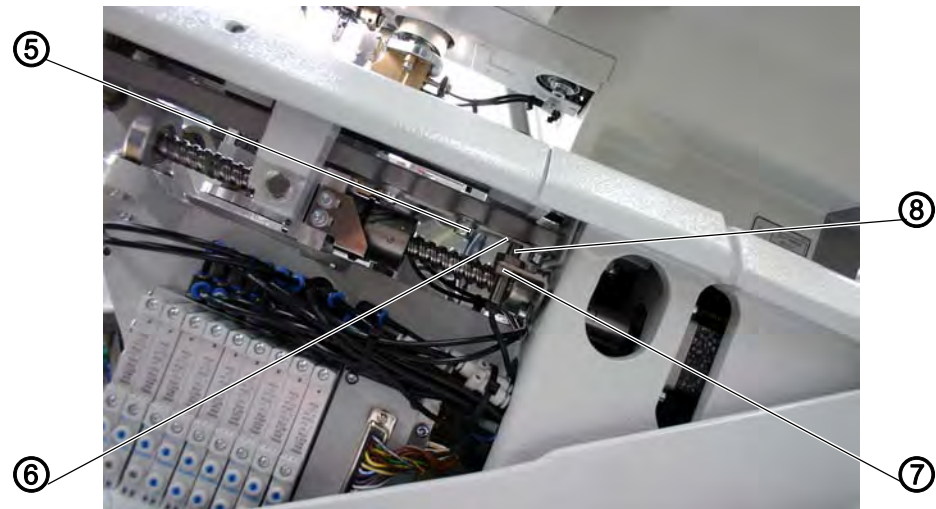
Fig. 21: Fabric support plate, setting the transverse movement (2)
