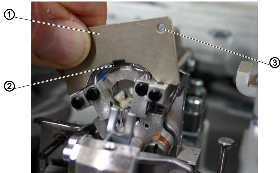
Fig. 63: Setting the looper height
