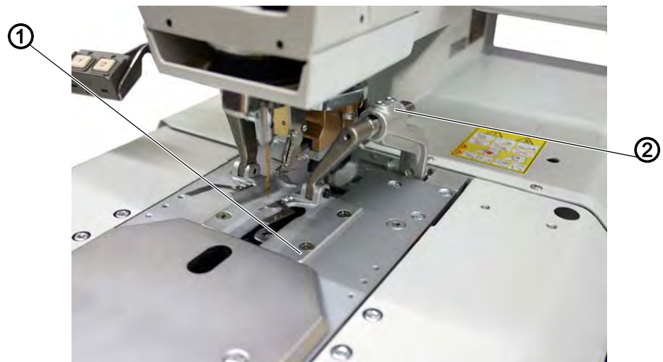
Fig. 35: Latching the clamping plates (1)
