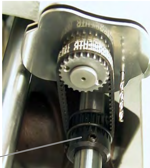
Fig. 6: Setting the thread take-up disk (3)
