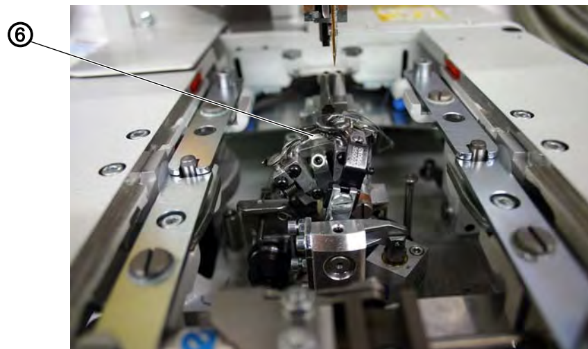
Fig. 81: Setting the needle thread blade (3)
