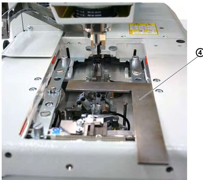
Fig. 15: Aligning the looper turret (4)
