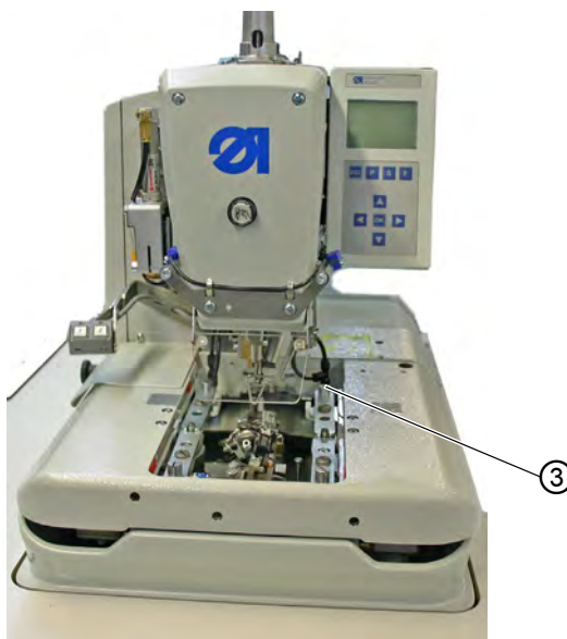
Fig. 35: Fitting clamping plates
