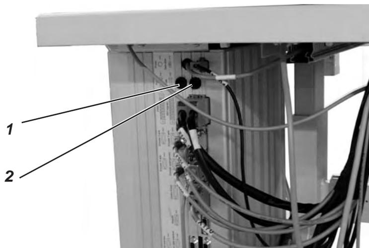
The fuses 1 and 2 for the control are on the back of the control box. Only insert the fuses indicated in the circuit diagram.
