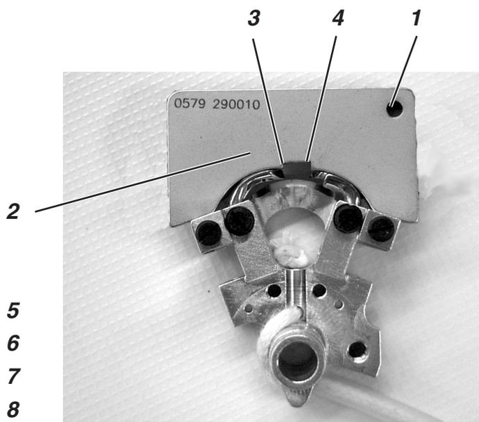
Before the setting of the looping stroke and the needle bar height and particularly after needle breakage, the correct looper height must be checked.
