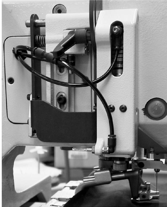
With the exception of subclass 579-151000, all subclasses have a needle thread catcher as standard equipment. The subclass 579-151000 can be retro-fitted with the needle thread catcher, if desired.
