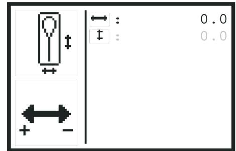
The position of the knife can be corrected in this menu. The position of the knife can be corrected by  $\pm 0,3$  mm on both axes. Which direction is meant by “+” and “-” is shown in the symbol at the lower left in the display.
