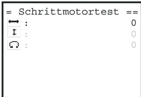
The step motors for the three motion axes of the 579 can be tested in this menu.
