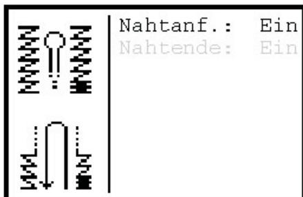
The stitch condensation at the seam beginning and seam end are turned on and off in this menu.
