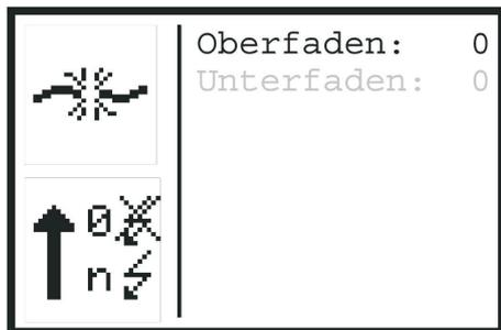
The thread monitors for the looper thread and the needle thread can be set in this menu. The values behind the needle thread and looper thread mean the following:
