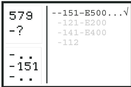
The subclass can be set in this menu. With the subclasses 579-112000 and 579-151000, the E-group can also be set. With the subclass 579-141000 the cutting length group can be selected.
