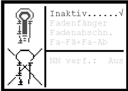
With the aid of the “Sewing Process” testing program, the switching order of the valves can be checked. This testing program is particularly helpful for the setting of the thread catcher and the thread trimming systems because one can see precisely how the individual components lie in regard to the needle thread, looper thread and the gimp.
