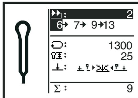
In the service menu of the 579, several base settings of the automatic sewing machine can be made and a number of test programs conducted. No maintenance or final position tasks are to be undertaken in the service menu.
