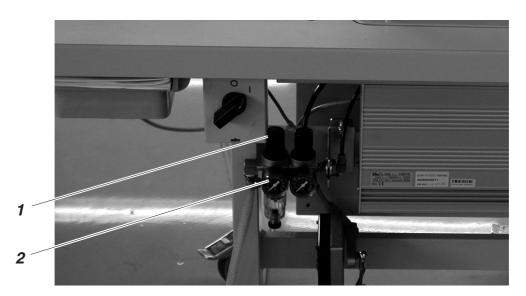
The pneumatic system of the machine and its auxiliary equipment must be supplied with compressed air containing absolutely no water or oil.
