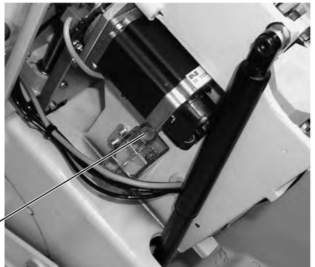
Check the oil level in the oil reservoirs 4 and 5 weekly !
