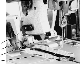
Through the spring-mounted clamp frame 2 found under the material support plate the pressure of the upper cloth clamps is automatically adjusted to the material thickness.
