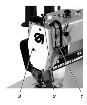
The pneumatically raised sewing foot can be arrested in the high position with button 3 (e.g. for winding the hook thread).
