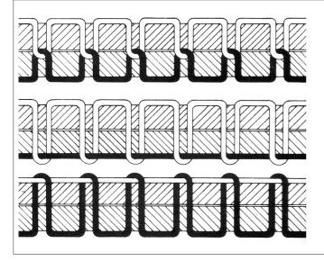
Illus. A: Correct thread interlacing in the middle of the material
