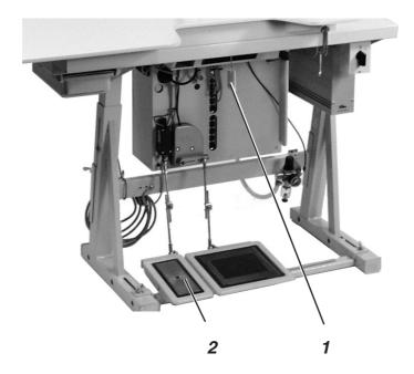
With the knee switch 1 one moves from one program step to the next in the sewing programs.
