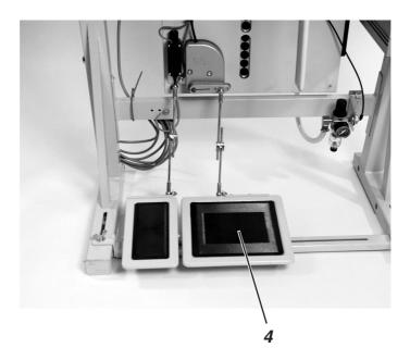
The sewing foot can be lifted pneumatically by operating the pedal 4.
