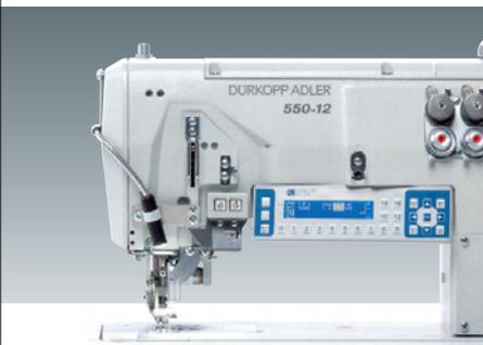
The optimized workstation with edge trimmer ensures a high rationalization effect by joining and ruffling of cover pieces and padding materials with simultaneously trimming of excess material. Precise trimming results, even with voluminous fillers and intensive ruffling, are guaranteed by the solid edge trimmer with high knife stroke and pulling cutting movement. This workstation can also be equipped with an ergonomically positioned lisier tape guide.
