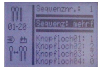
If *Sequence: multiple* is selected, you can select up to 20 buttonhole programs in the bottom half of the display. The display shows 4 buttonhole programs at a time.
