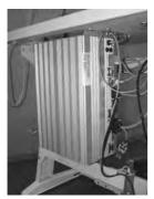
Mount the control unit (DAC III) onto the table plate using 4 wood screws according to figure 2 on page 10. The side with the bushes for the motors (three bushes, one under the other) has to point to the right side.
