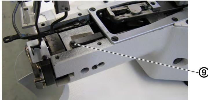
(9) - Connecting rod pin for needle thread clamp
