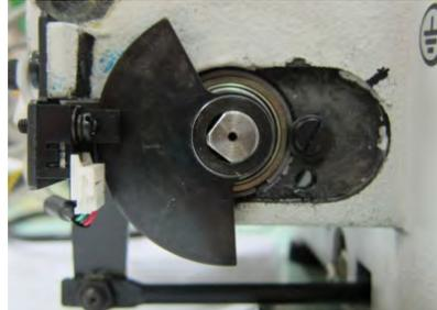
5. Check to see if the hole of the thread puller blade and the needle guide of the throat plate are aligned:
