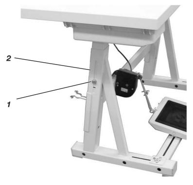
The working height can be set between 750 and 950 mm (measured up to the upper edge of the table plate).
