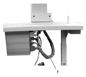
So that the top part of the machine can be folded back the leads coming from the top through the hole in the table plate either to the 15 gang multiple socket on the control box or to the cable channel must be long enough. To do this the leads must be laid in a large curve 1 using the cable ties.
