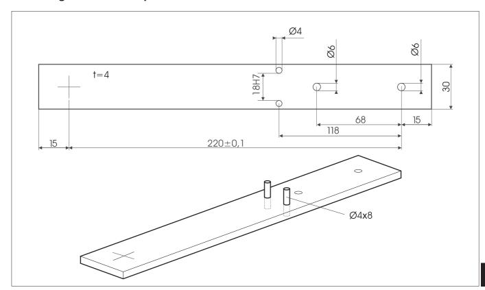
For setting the reference position the gauge shown above is required. The gauge cannot be ordered from Dürkopp Adler.
