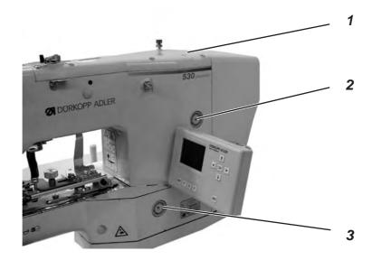
The button sewing automat is equipped with a central oil wick lubrication. The bearings are supplied by the oil reservoirs 2 and 3.
