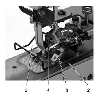
Some of the adjustments at the arm shaft 1 can be carried out easier if the thread trimming mechanism 3 is removed before.
