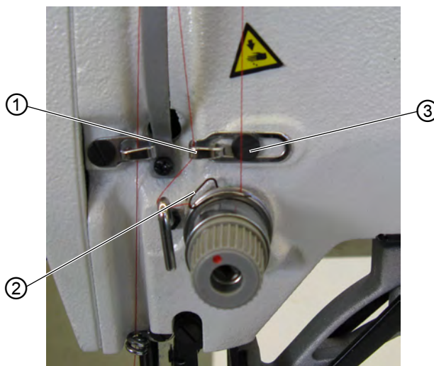
Fig. 3: Setting the thread regulator
