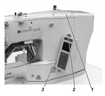
The automatic bartacker is equipped with central oil wick lubrication. The bearings are supplied by the oil reservoirs 2 and 3.
