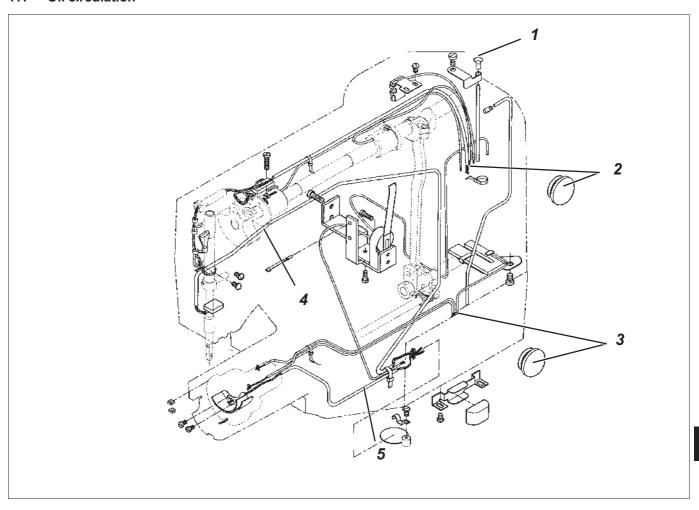
From the filler pipe 1, the oil flows into the oil reservoir 2 and then it runs over into the oil reservoir 3.
