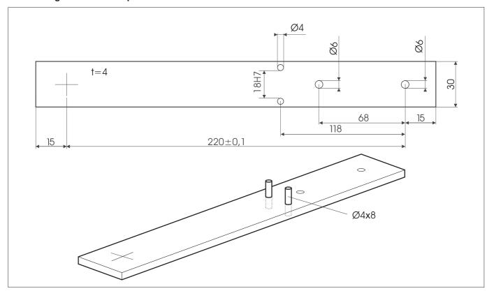
The gauge shown above is required for setting the reference position. The gauge cannot be ordered from Dürkopp Adler.
