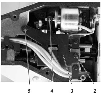
Some of the adjustments at the arm shaft 1 are easier to carry out if the thread trimming mechanism 3 is removed.
