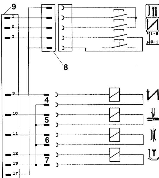
**Wiring diagram of connecting the electric elements of the machine head.**
