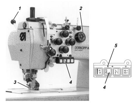
The feed distance of the roller top feed is a max. 7 mm.
