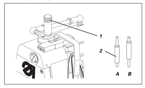
The desired sewing foot pressure is set with sleeve 1.
