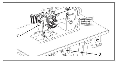
The sewing feet can be raised mechanically or pneumatically. Depending on the equipment of the special sewing machine, the lifting occurs through operation of the knee lever 2 or the stepping back on the pedal.
