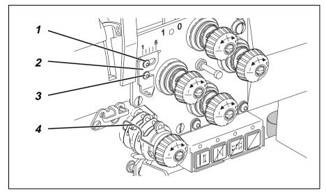
The needle thread quantity required for the hook is adjusted with the tension regulator 2.
