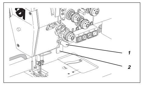
The needle bars can be turned off with lever 1.
