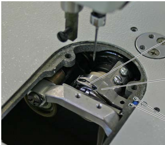
Figure. 29: Setting the counter-blade
