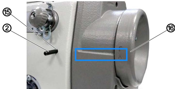
(2) - Locking peg (locking peg 3
