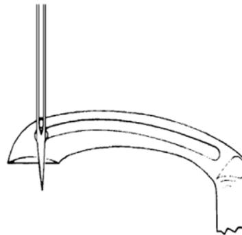
Fig. 74: Setting loop stroke and needle bar height (2)
