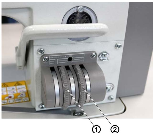
(1) - Adjusting wheel (for stitch length during bottom feed)
