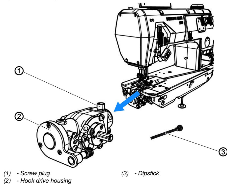
Fig. 124: Lubricating the hook (2)
