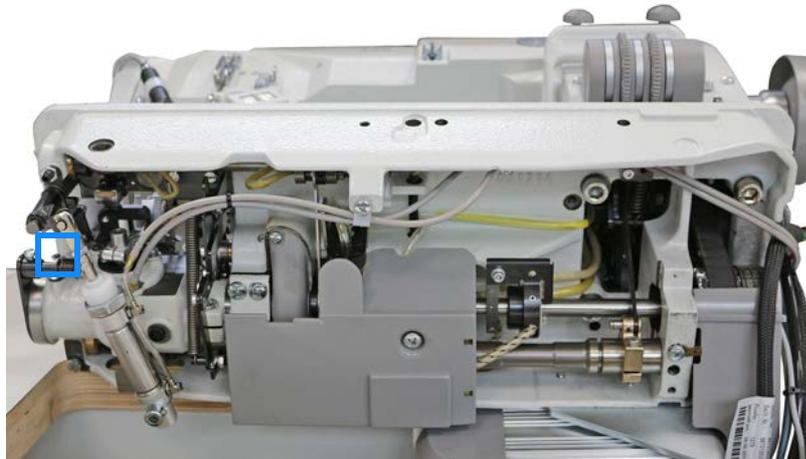
Fig. 78: Setting the needle guard (2)
