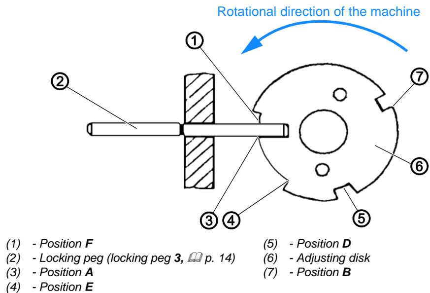
Fig. 26: Setting the adjusting disk relative to the arm shaft crank (2)
