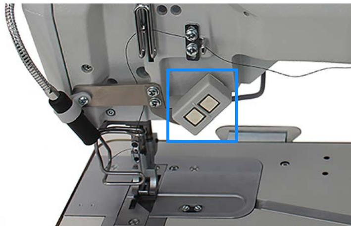
The two buttons on the push button panel can be assigned different functions. Possible function assignments are:
