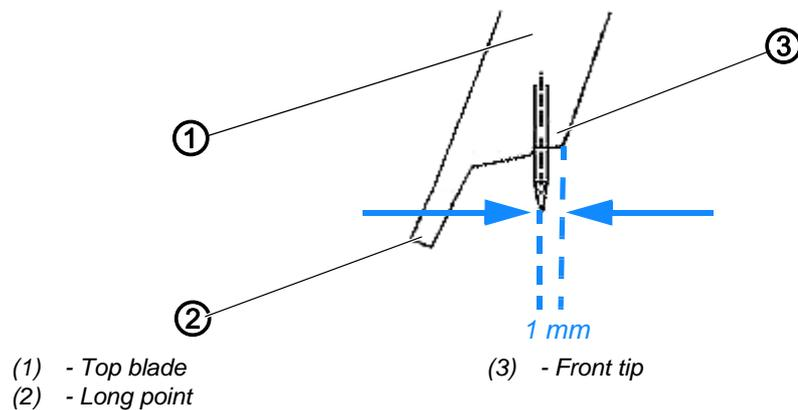
Fig. 113: Setting the height and lateral position of the top blade (2)
