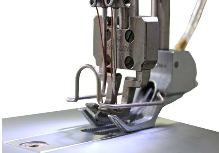
Fig. 2: General information: pneumatic seam middle guide in presser foot
