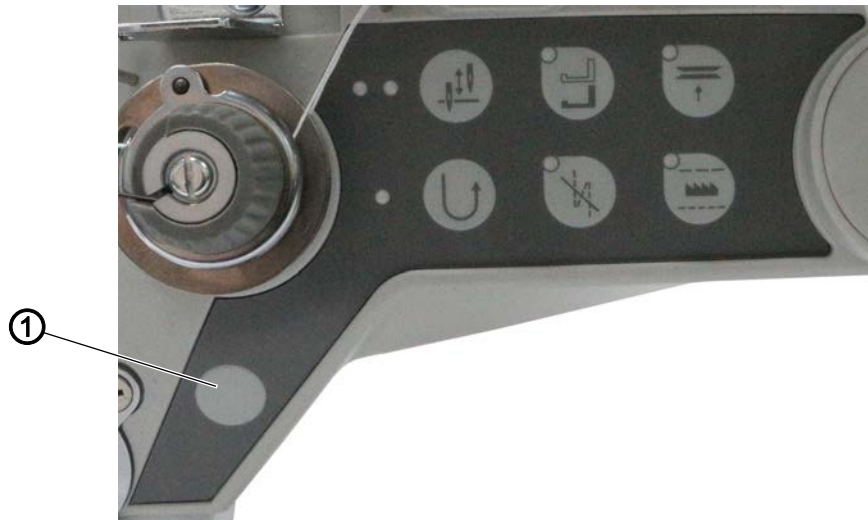
Fig. 14: Assigning bartack function to the Favorites button
