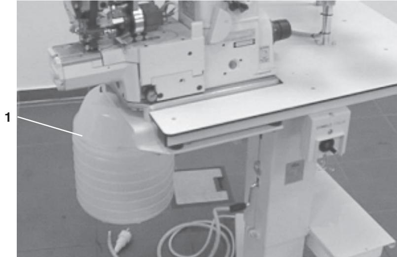
The cloth cut by the pinking mechanism and cut threads are collected in this basket.
