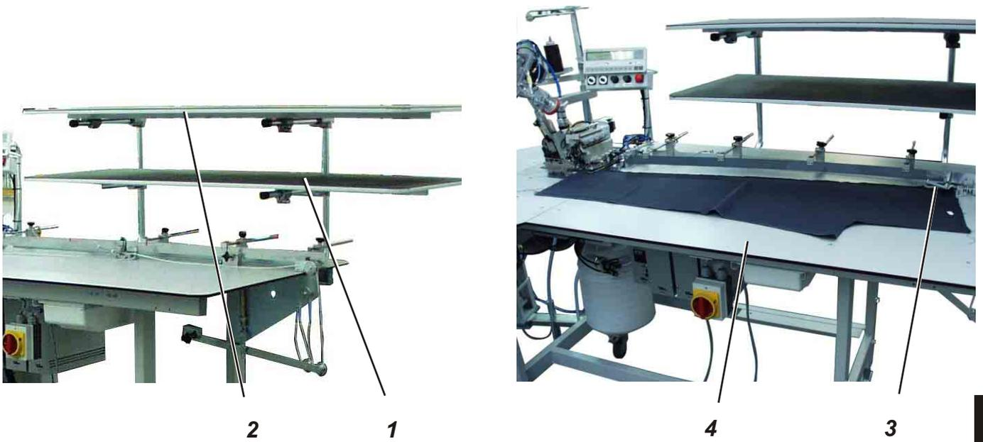
The sewing unit is equipped with two preparation tables 1 and 2. The skirt parts or trousers parts are positioned on them.
