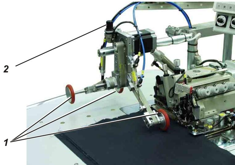
The pressure of the puller rollers 1 can be influenced via turning knob 2.
