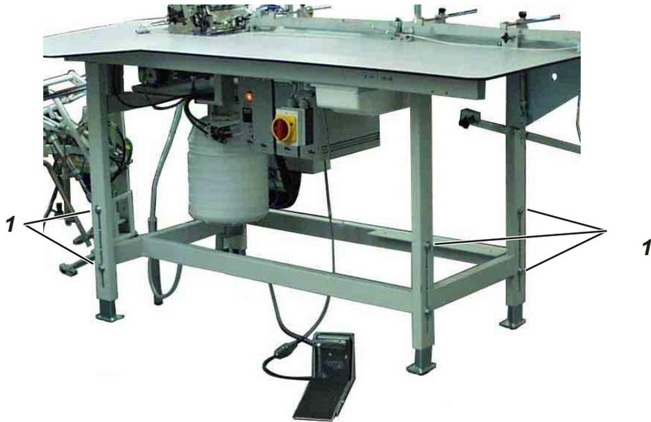
The working height is adjustable between 850 and 1200 mm (measured up to the top edge of the table top).
