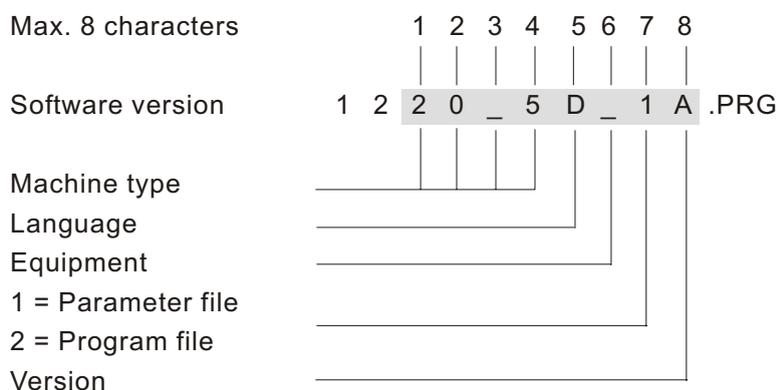
If different program or parameter files are stored, the control allocates a new name each.
