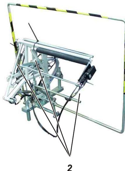
Before the installation of the sewing unit all transport protections have to be removed.
