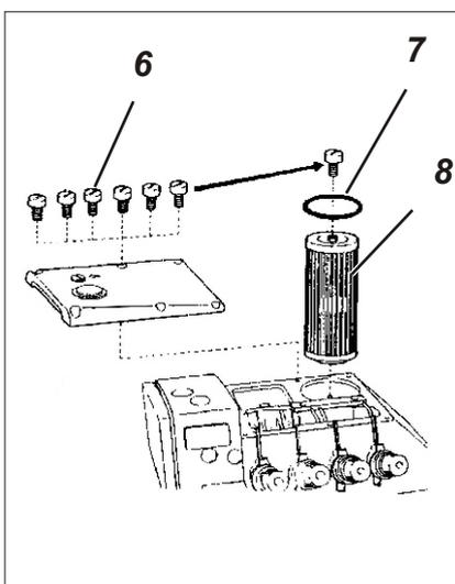
4 weeks after the initial start-up and subsequently every two years an oil change has to be carried out with the machine head disassembled.
