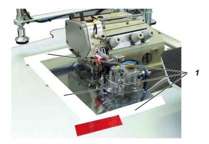
Before the installation of the sewing unit all transport protections have to be removed.
