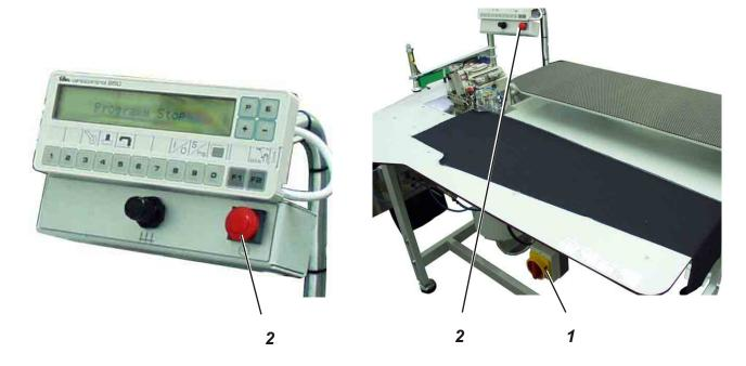
For an immediate stop in case of operating errors, needle breakage etc. the safety system of the machine provides the following measures:
