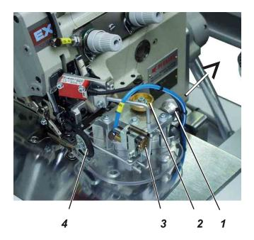
The height-adjustable edge guide ensures a precise positioning of the trousers part in front of the sewing head. The height of the edge guide can be adjusted according to the thickness of the material to be sewn.
