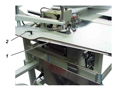
By means of the guide blade 1 the run of the workpiece can be influenced.
