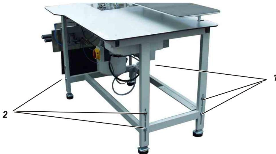
The working height is adjustable between 850 and 1200 mm (measured up to the top edge of the table top).
