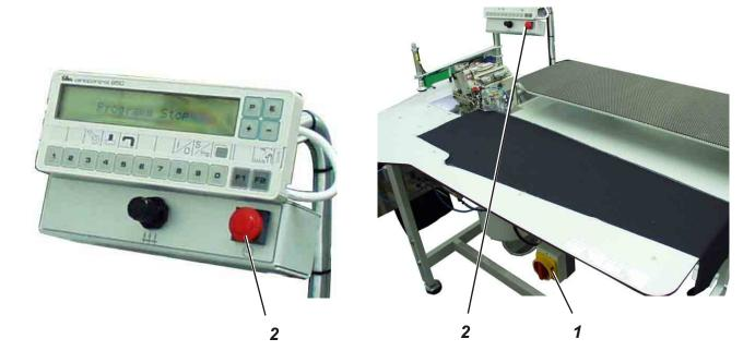
For an immediate stop in case of operating errors, needle breakage etc. the safety system of the 1220/5 provides the following measures:
