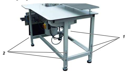
The working height is adjustable between 850 and 1200 mm (measured up to the top edge of the table top).
