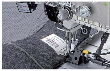
Class 550-867 – Identification of Endlabel-Barcode with all relevant information of the complete sewing process
