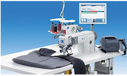
Dürkopp Adler has developed the new engineered sewing station 550-867 to realize these airbag tearing seams in a professional way.
