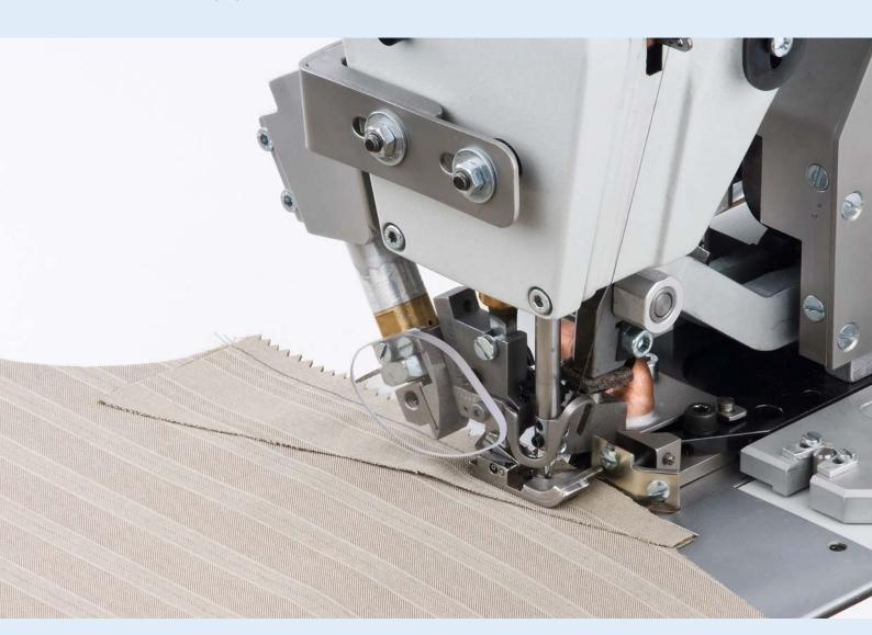
Attaching and pinking the crotch gusset – efficient working method
