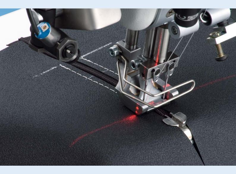
Displacement-free inserting of zippers
